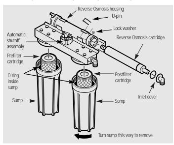
Reverse Osmosis Cartridge—The cartridge, inside the Reverse Osmosis housing, includes a tightly wound, special membrane. Water is forced through the cartridge where the membrane removes the dissolved solids and organic matter. High quality product water exits the Reverse Osmosis housing and goes to the storage tank. Reject water, with the dissolved solids and organic matter, leaves the housing and is discharged to the drain through 1/4" tubing.
