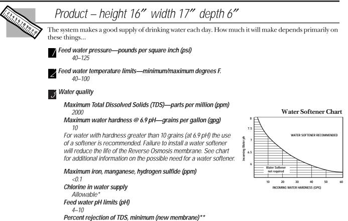
\*Chlorine removed (maximum of 2.0 ppm) by the Reverse Osmosis prefilter...regular changing of the prefilter is required. Chlorine will destroy the Reverse Osmosis membrane.
