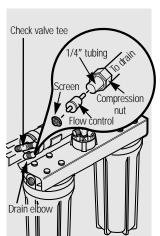
*Flow Control and Screen* The flow control regulates the flow of water through the Reverse Osmosis cartridge at the required rate so high quality product water is produced.
