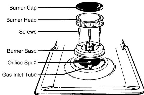
1. Remove grates, burner caps and burner heads.
