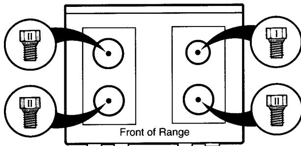
**Orifice Spuds for Converting to Natural Gas:**
