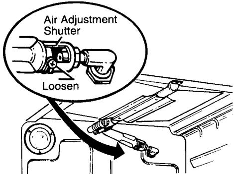
The air adjustment shutter for the top (broil) burner is in the center of the rear wall of the oven. (See Installation Instructions in this book.)
