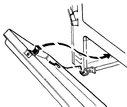
**To replace**, insert the two slots at bottom of panel onto the two tabs at base of range and push top of panel forward to engage spring clips.
