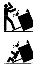
If you pull the range out from the wall for any reason, make sure the Anti-Tip device is engaged—when you push the range back against the wall.
