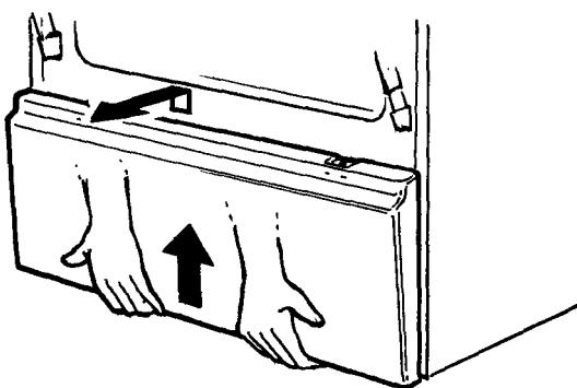
**To remove**, lift up bottom of panel slightly to disengage the panel from the tabs at the base of the range. Pull bottom of panel forward until spring clips are released at top of panel.
