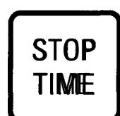
"5:00" appears on the display and "STOP TIME" flashes. The control automatically sets Stop Time by adding the Cook Time to the time of day. In this example, the time of day is 2:00 and the Cook Time is 3 hours. Adding 3 hours to the time of day equals 5:00.
