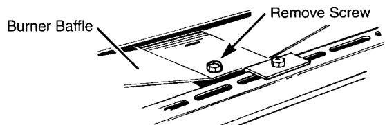
To remove the burner baffle (on some models):
