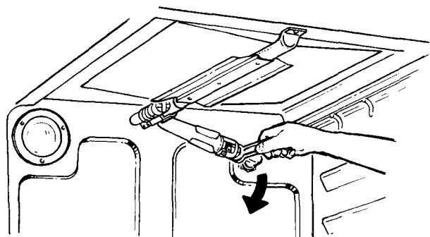
**To convert to LP gas,** use a 1/2" wrench to turn the upper burner orifice spud clockwise. Tighten spud only until it is snug with the base. To prevent damage, do not overtighten spud.
