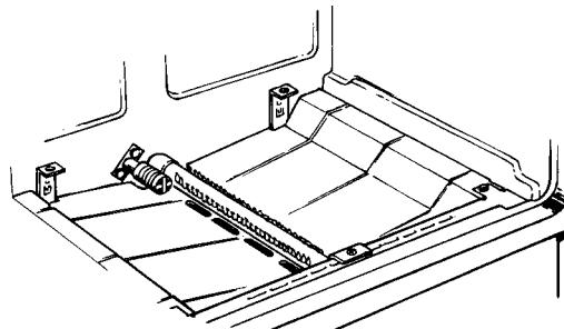
The flames should have 1/2" to 3/4" blue cone with no yellow tipping. When the baffle is back in place, the flames will resettle.
