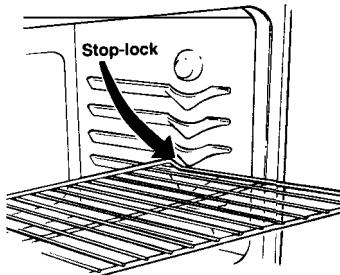
When placing cookware on a shelf, pull the shelf out to the "stop" position. Place the cookware on the shelf, then slide the shelf back into the oven. This will eliminate reaching into the hot oven.
