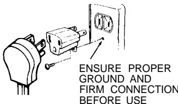
**CAUTION:** Attaching the adapter ground terminal to the wall receptacle cover screw does not ground the appliance unless the cover screw is metal, and not insulated, and the wall receptacle is grounded through the house wiring. The customer should have the circuit checked by a qualified electrician to make sure the receptacle is properly grounded.
