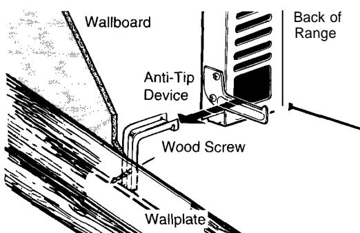
5. Slide the range against the wall, and check for proper installation by grasping the front edges of the rear surface unit openings and carefully attempting to tilt the range forward.
