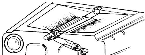
The flames for the top (broil) burner should be steady with approximately 1" blue cones and should not extend out over the edges of the burner baffle.
