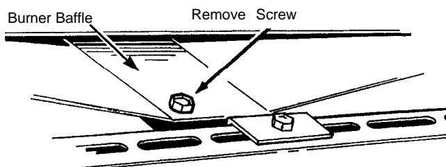
**To remove the burner baffle**, use a nut driver to remove the 1/4" hex head screw shown in the illustration above. Do not remove any other screws. Pull baffle straight out until it is free from the slot that holds it at rear of oven.
