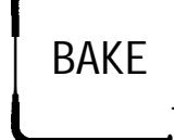
**Step 7:** Press INCREASE pad. The last oven set temperature appears in the display. Press INCREASE or DECREASE pad until "325" is displayed.
