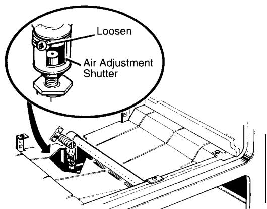
The shutter for the bottom (oven) burner is near the back wall behind the storage drawer or the kick panel (depending on the model). Remove the drawer or panel. (See Care and Cleaning section in this book.)
