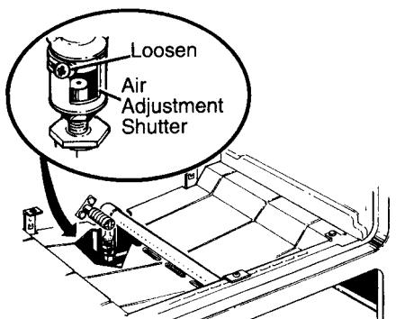
The shutter for the bottom (oven) burner is near the back wall behind the storage drawer, or kick panel.
