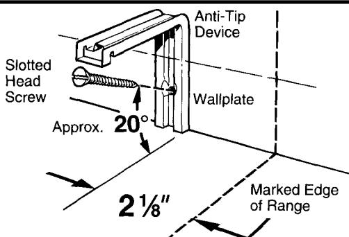
2. Locate the outside edge of the device 2%" toward the center of the range from the marked edge of the range.
