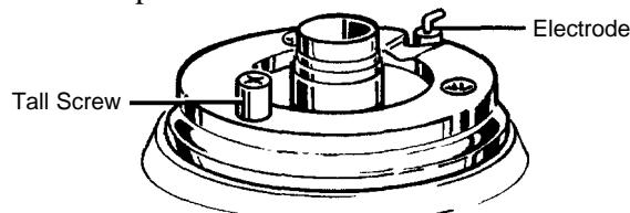
7. Carefully insert burner bases straight down with the tube over the orifice spud. Replace the screws, **making sure the tall screw is opposite the burner electrode in each burner base.**
