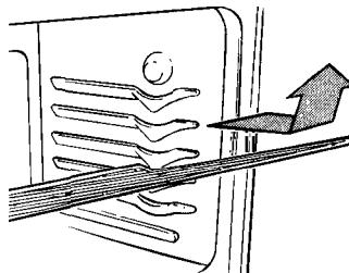
To replace, place shelf on shelf support with stop-locks (curved extension of shelf) facing up and toward rear of oven. Tilt up front and push shelf toward back of oven until it goes past "stop" on oven wall. Then lower front of shelf and push it all the way back.
