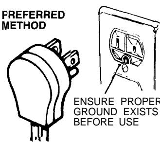
qualified electrician to make sure the receptacle is properly grounded.
