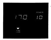
**4.** Finished temperature reached. A 3 second signal sounds and the oven shuts off automatically.
