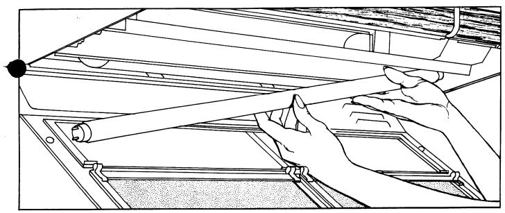
To replace hood lamp, first disconnect power at main fuse or circuit breaker panel or pull plug. Remove 2 screws from each side of lower panel and 3 screws from front edge. Lower panel until it rests on range below. Place fingers on top near each end of lamp. Press down and roll top of lamp gently toward
