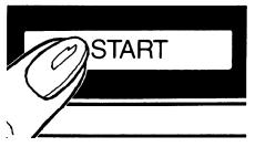
**Step 4:** Touch START. Inside light comes on and fan starts. Cooking time counting down shows on display.
