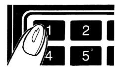
Step 3: Select your time. Touch 1, 2, and 0 for a minute and 20 seconds. Readout shows 1:20. If another Power Level is desired touch Power Level and the number although Power Level 10 (HIGH) is preferred for this cup of coffee.
