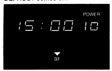
Step 2: Touch 1, 5, 0, and 0 for defrosting time. 15:00 and Power 3 appear on readout. (Defrosting is automatically set on Power Level 3 but can be changed by touching POWER LEVEL pad and the new Power Level.)
