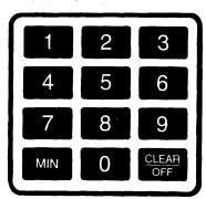
**3.** CHANGE POWER LEVEL if you want a Power Level other than automatic 10 (cooking) or 3 (defrosting). Touch Power Level pad, then number pad needed.
