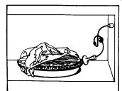
1. Insert Probe and insert cable end into receptacle. Touch **TEMP COOK**.
