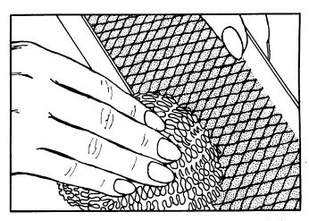
Soak, then agitate filter in hot detergent solution. Don't use ammonia or other alkali because it will darken metal. Light brushing can be used to remove inbedded dirt. Rinse, shake and remove moisture before replacing. Filters should be cleaned at least once a month. Never operate your hood without the filter in place. In situations where flaming might occur on surfaces below hood, filter can retard entry of flames into the unit.
