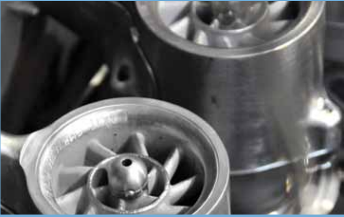
Premixers with double counter-rotating swirler
