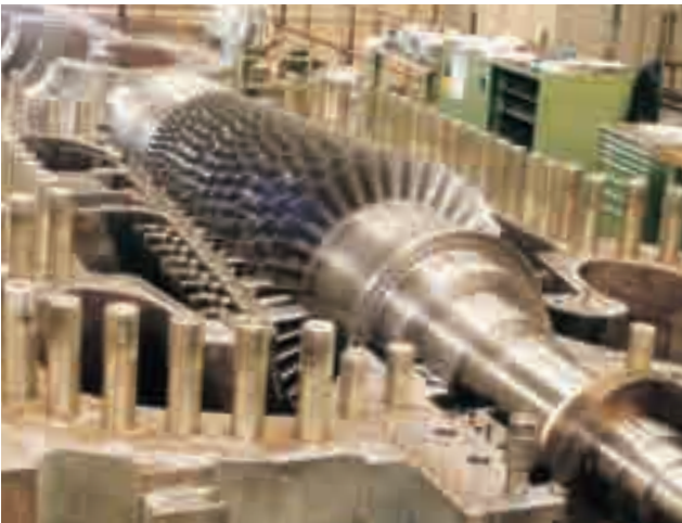
Mixed Refrigerant Compressor for LNG Plant
