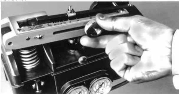
Figure 4 - Adjusting the C_v of VariPak 28002 valve for each plug/seat ring combination
