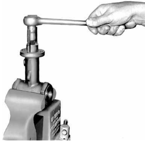
Figure 19 - Tightening the seat-ring retainer (4)
