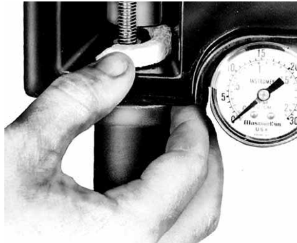
Figure 18 - Adding a packing ring
