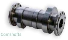
The camshafts on the L250 are made of sectional carbon steel forgings joined by dowel-bolted flanges, a design that simplifies component removal and replacement. Individual sections of the camshaft, rather than the entire camshaft, can be serviced or replaced.
