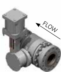
Figure 5.1 Mount #1 - Left Hand (Standard) with clean sweep feature Actuator located on left hand side of valve when looking in direction of flow (actuator vertical/valve stem horizontal).
