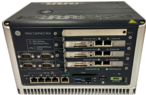
Visor Connect Box, providing a unified interface to GE Power Conversion site equipment
