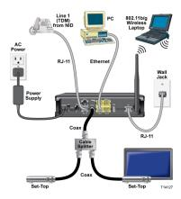
For IPTV service, you must connect the residential gateway to an IP set-top. You can connect to an IP set-top using an Ethernet or coaxial connection.
