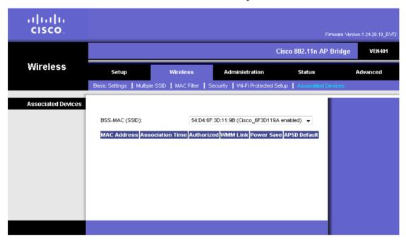
To view details for an associated device, select the SSID from the drop-down menu. The page refreshes with a list of devices associated with the selected SSID and general information for each device found.
