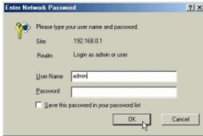
In order to configure the WX-2211 you must input the user-name into the **User Name** box. Enter the password into the **Password** box and press the **OK** button. The default User Name is “admin”. There is no default password, leave the Password field blank.
