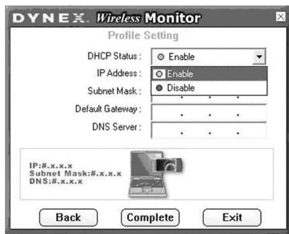
The purpose of this screen is to configure the TCP/IP setting of each wireless connection. You must define if the current profile's IP setting is assigned by a DHCP server or assigned by a fixed IP that is determinate by the Network Administrator.
