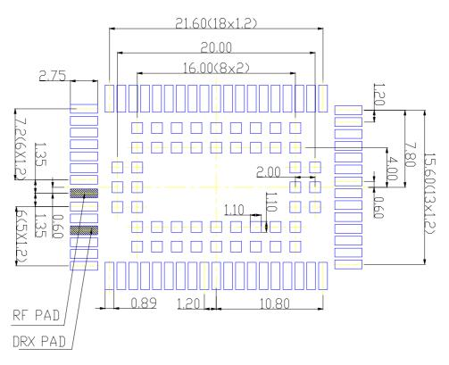
Figure 44: Recommended design for 120 micron thick stencil (top view, dual design)
