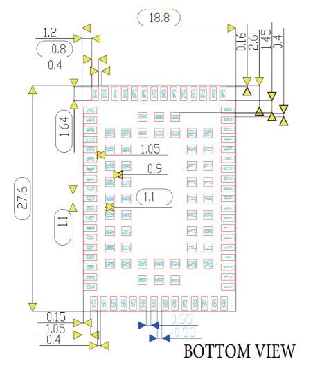
Figure 42: Dimensions of ELS31-VA/ELS51-VA (all dimensions in mm) - bottom view
