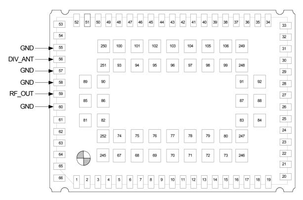
Figure 22: Antenna pads (bottom view)
