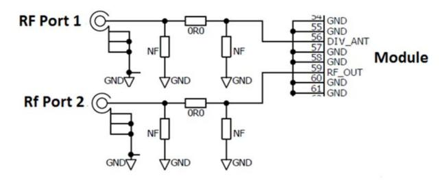
Figure 23: RF interface signals example
