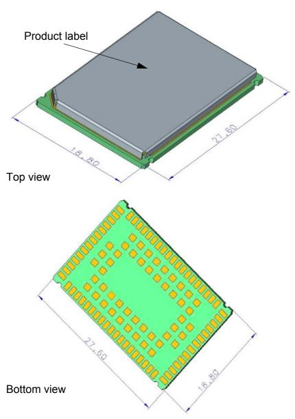
Figure 40: ELS31-VA/ELS51-VA- top and bottom view
