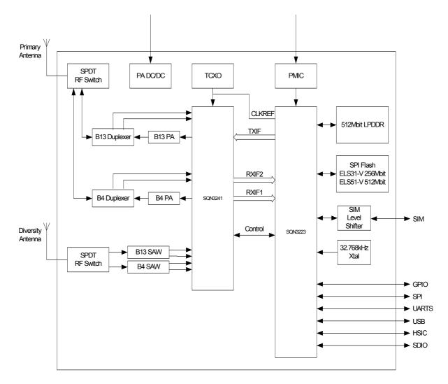
Figure 2: ELS31-VA/ELS51-VA baseband block diagram
