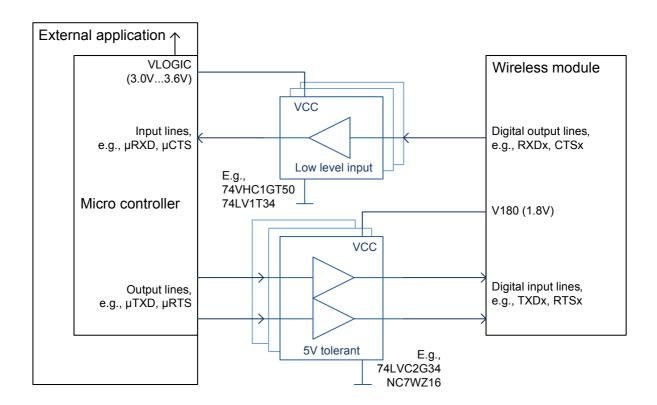
Figure 30: Sample level conversion circuit
