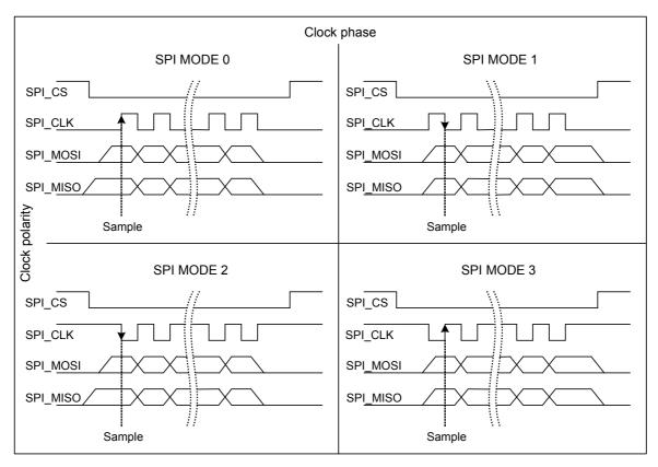
Figure 16: Characteristics of SPI modes
