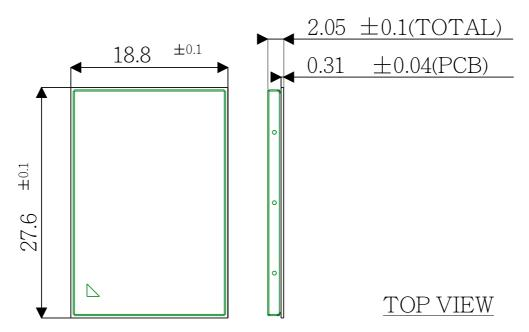
Figure 41: Dimensions of ELS31-VA/ELS51-VA (all dimensions in mm)
