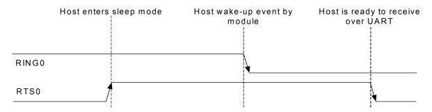
Figure 20: Wake-up via RING0
