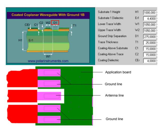
Figure 26: Micro-Stripline on 1.0mm Standard FR4 PCB - example 2
