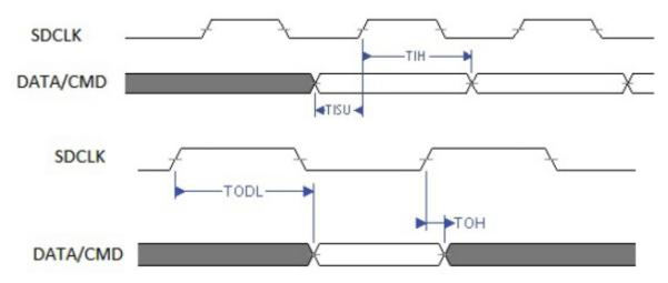
Figure 17: SDIO interface timing diagrams (Input/Output)
