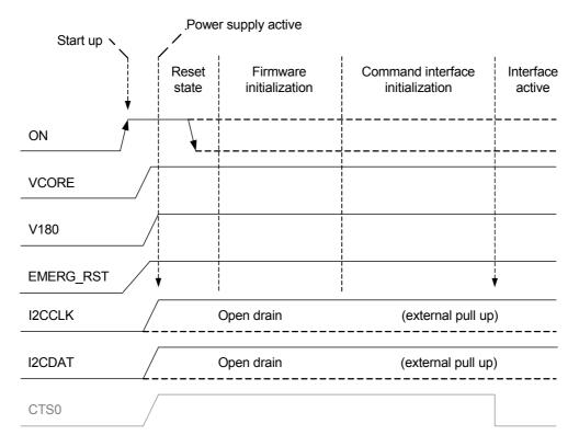
**Figure 15:** I<sup>2</sup>C startup behavior
