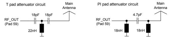
Figure 38: ESD protection for RF antenna interface
