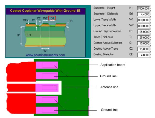
Figure 27: Micro-Stripline on 1.5mm Standard FR4 PCB - example 1
