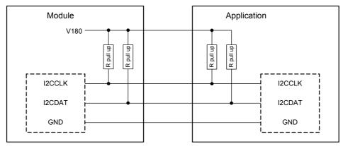
Figure 14: I<sup>2</sup>C interface connected to V180
