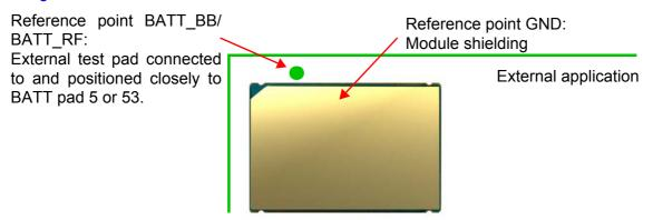
Figure 37: Position of reference points BATT\_BB/BATT\_RF and GND
