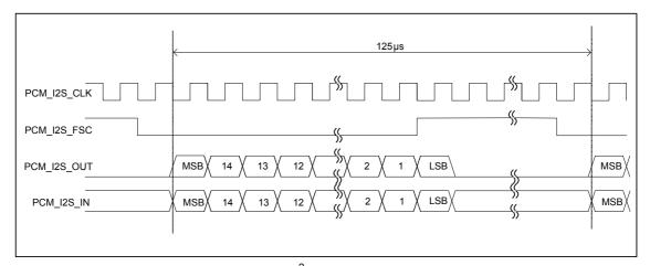
**Figure 12:** I<sup>2</sup>S timing (slave mode)
