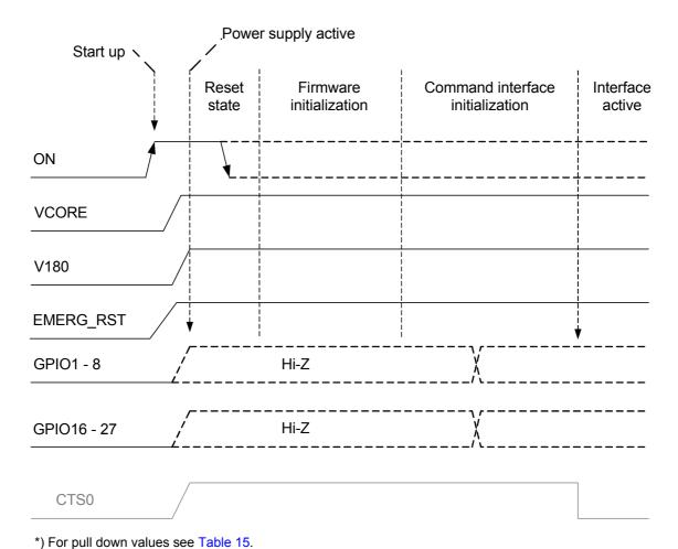
Figure 13: GPIO startup behavior
