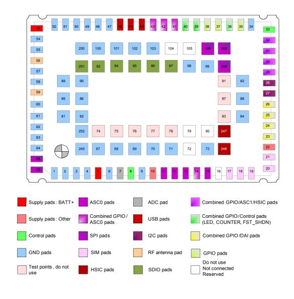
Figure 3: Numbering plan for connecting pads (bottom view)
