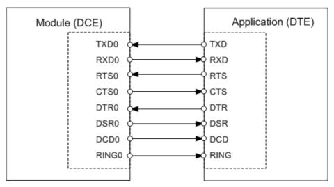
Figure 6: Serial interface ASC0
