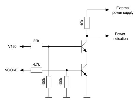
Figure 19: Power indication circuit
