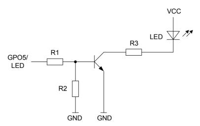
Figure 18: Status signaling with LED driver
