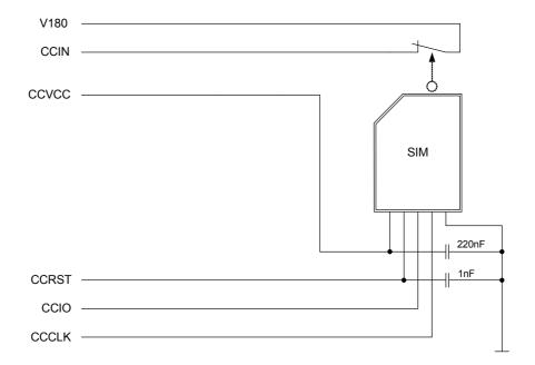
Figure 10: External UICC/SIM/USIM card holder circuit
