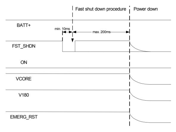
Figure 21: Fast shutdown timing
