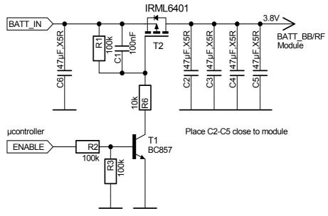
Figure 31: Sample circuit for applying power using an external μC
