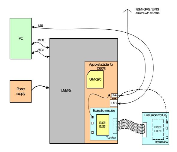
Figure 56: Reference equipment for Type Approval
