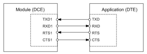
Figure 8: Serial interface ASC1
