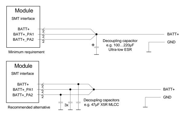
Figure 2: Decoupling capacitor(s) for BATT+
