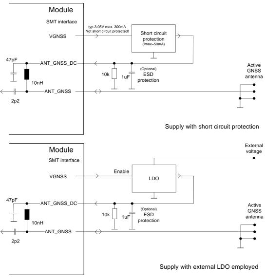
Figure 6: Supply voltage for active GNSS antenna
