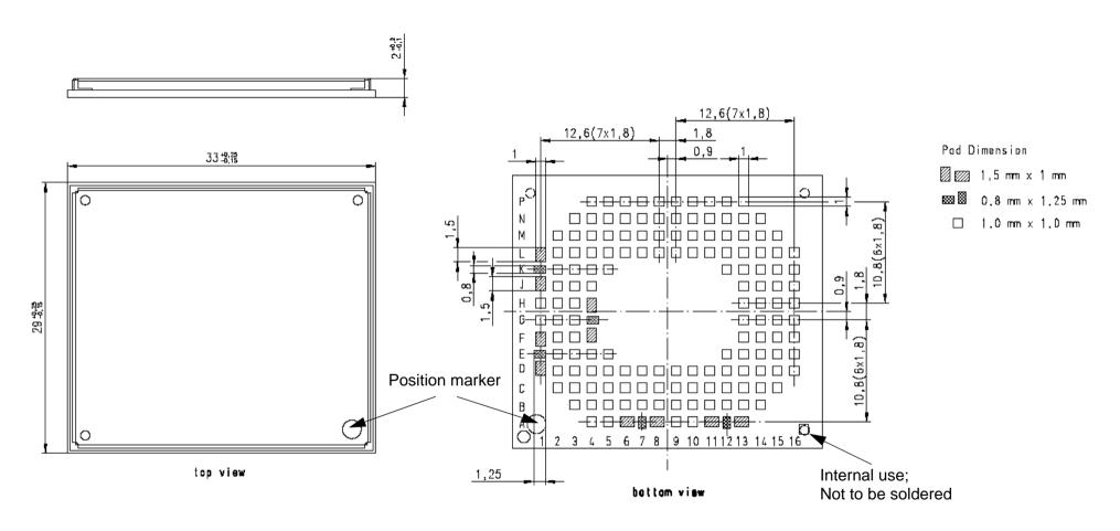
Figure 9: Dimensions of PXS8 (all dimensions in mm)
