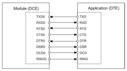
Figure 4: Serial interface ASC0
