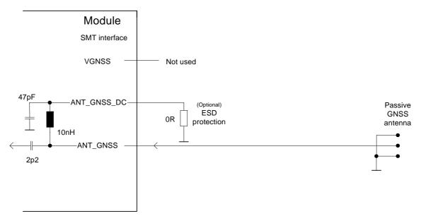
Figure 7: ESD protection for passive GNSS antenna
