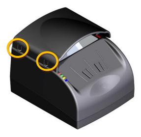
3. To re-attach the document hood, ensure that the pin on the right of the hood is correctly seated before pressing down on the tabs on the left of the hood.
