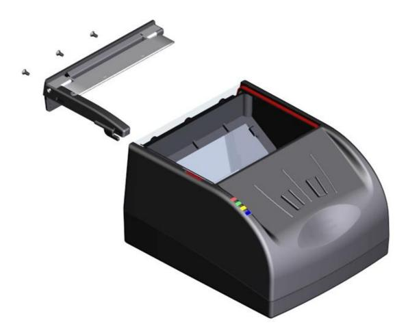
4. Gently slide the glass to the back of the reader while being careful not to damage or remove the rubber gasket seal.
