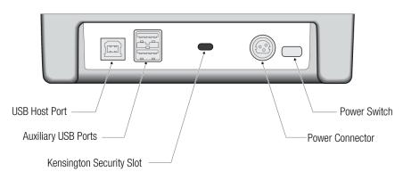
The reader is capable of operating on USB 2.0 power. However, when operating on USB power, due to the limited power available over the USB interface:
