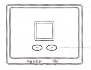
Press the ∧ or ∨ button once to display the setpoint temperature. The setpoint temperature will be displayed for 5 seconds. Press either button while the setpoint is displayed to change the setpoint.
