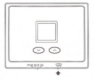
Use the Fan switch to select the fan operation.
