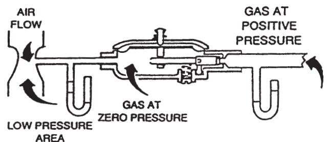
Figure 2.10 – LP Gas Carburetion Diagram
