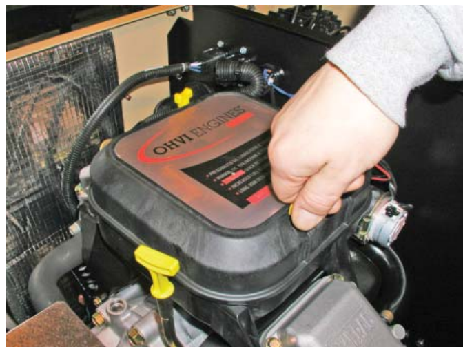
Figure 2.2 – Restrict Air Flow During Initial Start Up
