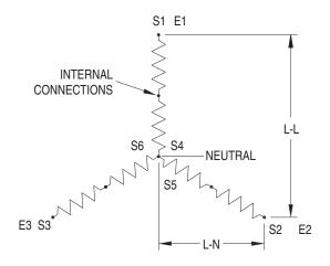
Figure 7.3 — Stator Power Winding Connections - 3-phase, 120/208V (6 Lead)
