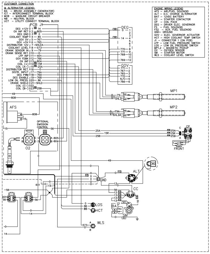
WIRING - DIAGRAM 2.4L 4 POLE
