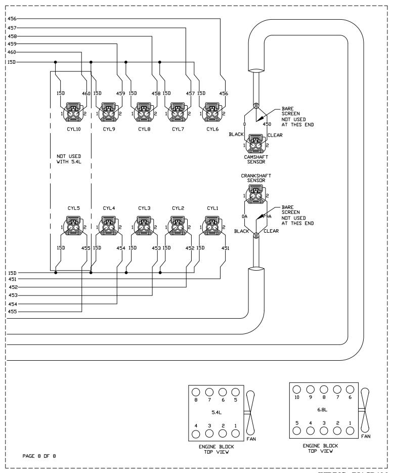
REVISION: G-6035-C DATE: 07/27/05 WIRING - DIAGRAM 5.4 & 6.8L H-PANEL DRAWING #: 0F2576
