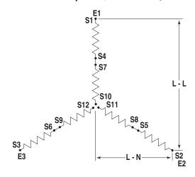
Figure 7.3 — Stator Power Winding Connections - 3-phase, 120/208V (12 Lead)
