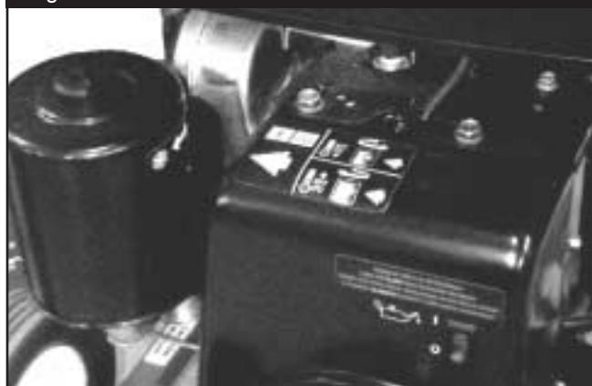
Figure 6 — Air Cleaner Position At or Below 32°F
