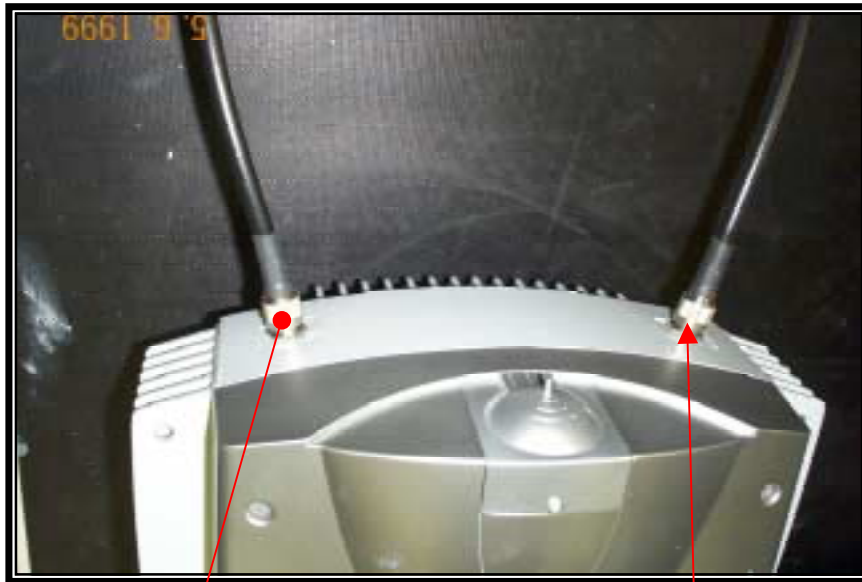
Main Antenna Tx & Rx – Left Hand Side
