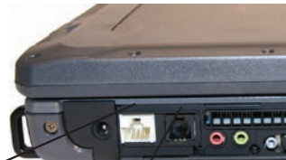
Ethernet Port (RJ45) Modem Port (RJ11)
