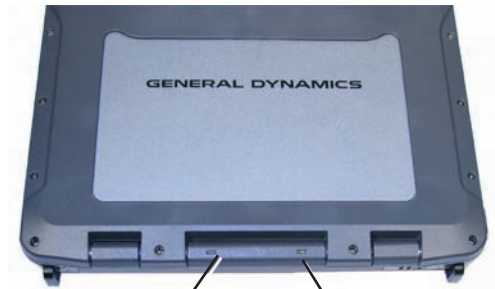
Wireless Modem LED Power LED
