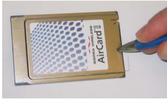
Figure 2-2: Ejecting the SIM card
