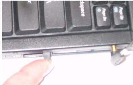
Figure 5-2: Ejecting the AirCard from its slot
