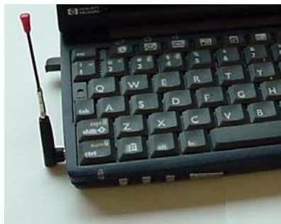
Figure 5-1: Proper positioning of the AirCard antenna
