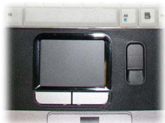
Resistive Touchpad option: works with gloved fingers
