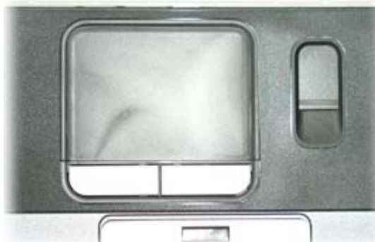
Capacitive Touchpad option: works well with fingers
