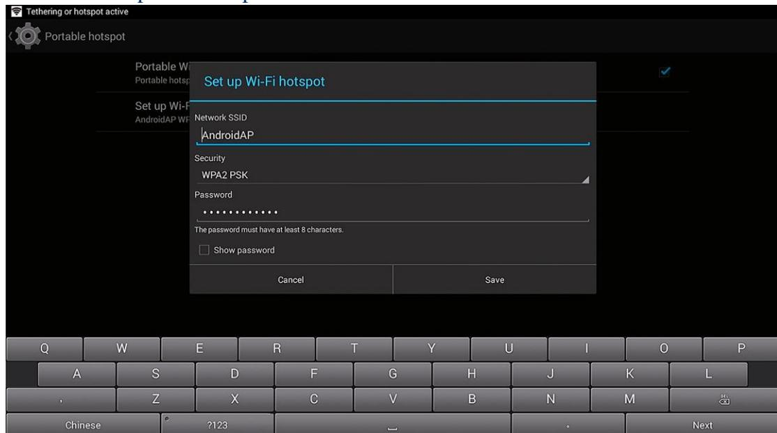
Note: WiFi and hotspot connection can not be applied at same time. Disconnect WiFi and connect Ethernet while using hotspot function.
