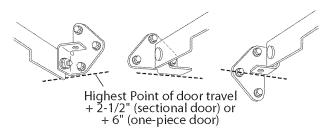
Figure 18 Attach Header Bracket above Garage Door
