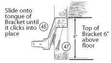
Figure 25 Install Safe-T-Beams®
