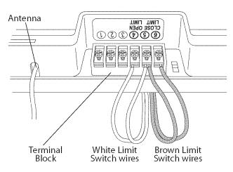
Figure 15 Connect Limit Switch Wires to Power Head Terminal Block
