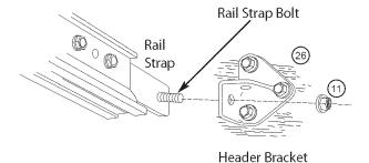
Figure 20 Attach Rail Strap to Header Bracket
