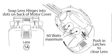
Figure 41 Install Lens Cover and Light Bulbs
