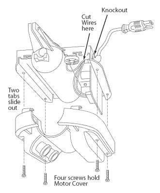
Figure 33 Connecting power with permanent wiring
