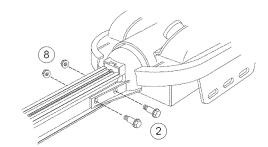
Figure 10 Bolt 1st Rail Section to Power Head
