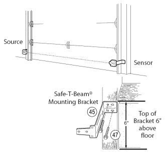
Figure 7 Mounting Safe-T-Beam® Components
