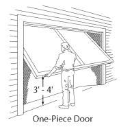
Figure 1 Checking door balance
