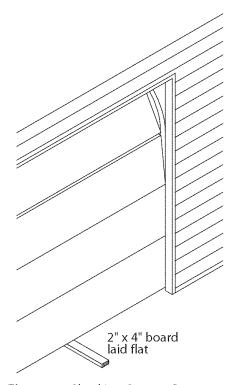
Figure 36 Checking Contact Reverse
