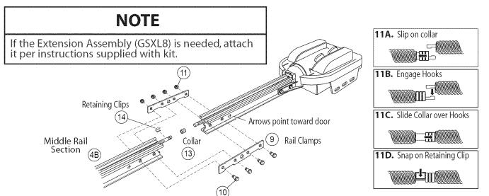
Figure 11 Attach Middle Rail Section
