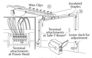
Figure 29 Wiring Method A
