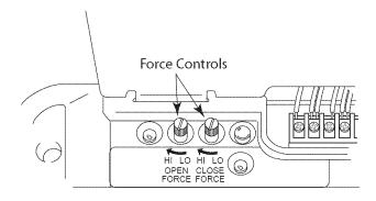
Figure 35 Making Force Adjustments
