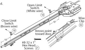
Figure 14 Install Limit Switches on Assembled Rail
