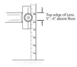
Figure 27 Final Check Safe-T-Beams®
