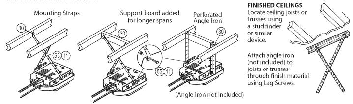
Figure 22 Mounting methods for open beam and finished ceilings
