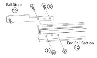
Figure 13 Attach Rail Strap
