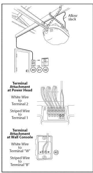
Figure 32 Install Wall Console with Entrapment Warning Label
