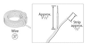
Figure 28 Wire the Safe-T-Beam® System
