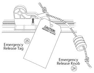
**Figure 16** Attach Emergency Release Cord/Knob and Tag
