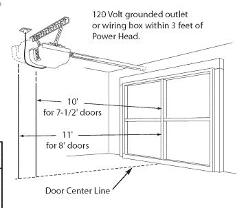
Figure 5 Check Power Head location
