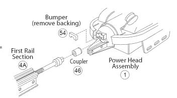
Figure 9 Install Bumper, Coupler and 1st Rail Section
