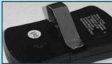
FIG. 8-3 Attach visor clip.
