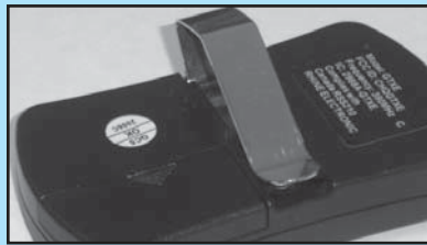
FIG. 8-3 Attach visor clip.
