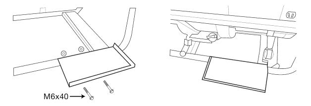
2) Put the battery on the frame, have the battery assembled with the provided accessories as shown.
