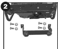
Here is the hardware required to install the support leg. Place a block of wood under the generator so that you don't have to hold it up while trying to install the leg.
