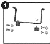
Start by installing the rubber floor mounts onto the support leg as shown. Note: The leg should be installed on the same side as the pull handle.
