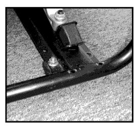
This generator has an option of not using the mobility kit. If this is desired, just install the 4 rubber mounts on the frame as shown. (this is why there are 6 mounts). If you want to use the mobility kit, save the 4 mounts in a safe place, and continue to the "mobility kit installation." section.
