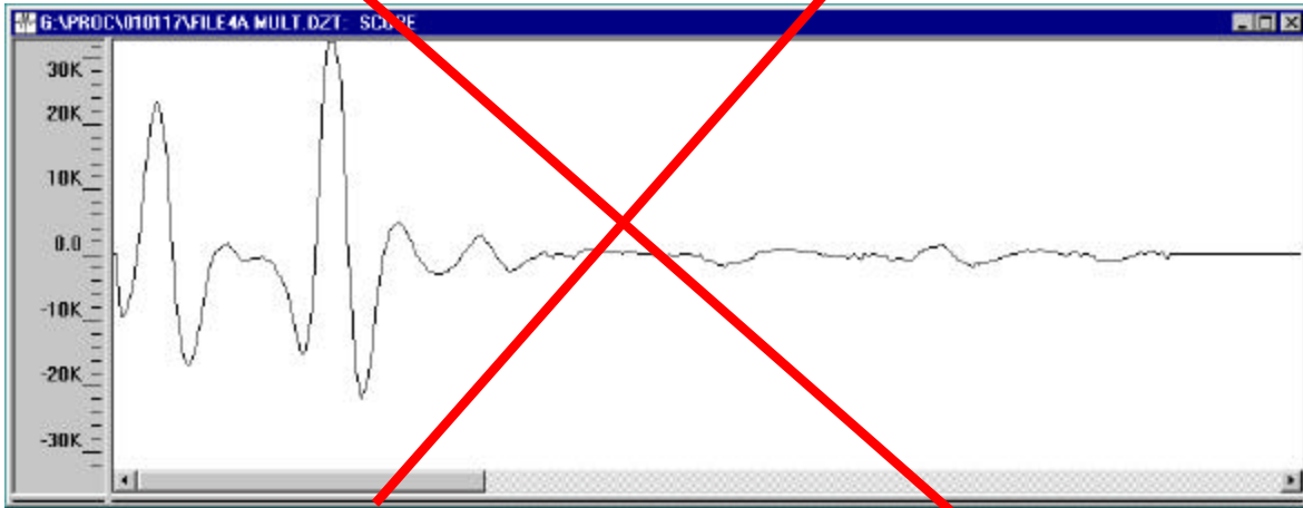
Figure 3: Example of Model 4108F data scan collected with too much gain.
