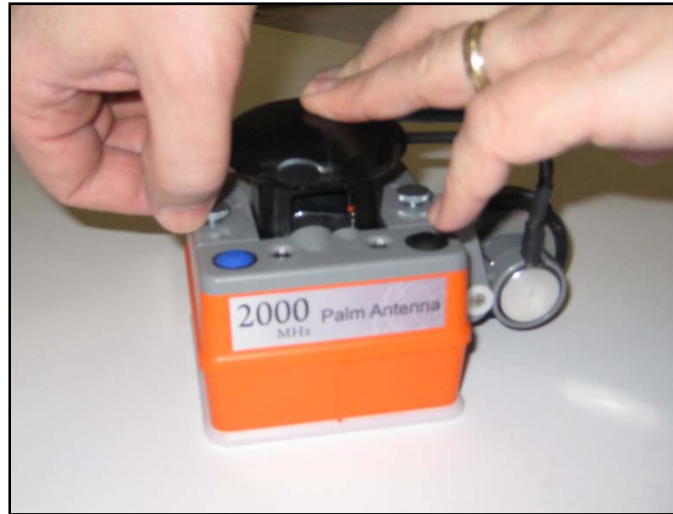
Figure 5: Re-secure the encoder assembly.
