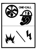
**WARNING:** Always contact your local One-Call system before the start of your digging project. The Interragator II GPS system is intended to be used with other utility locating methods, such as the use of the One-Call system and potholing.
