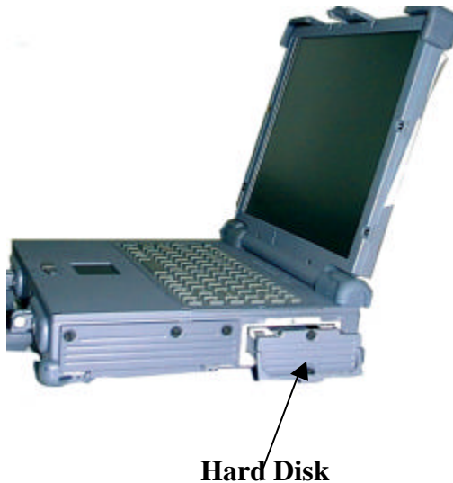
Figure 2-7 Removing a Hard Disk
