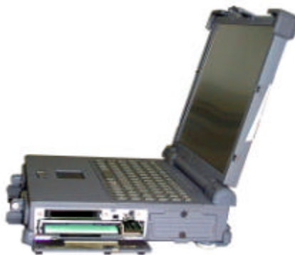
Figure 2-4 Removeing a Diskette
