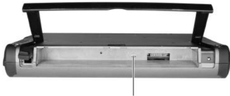
Backup Battery Switch
