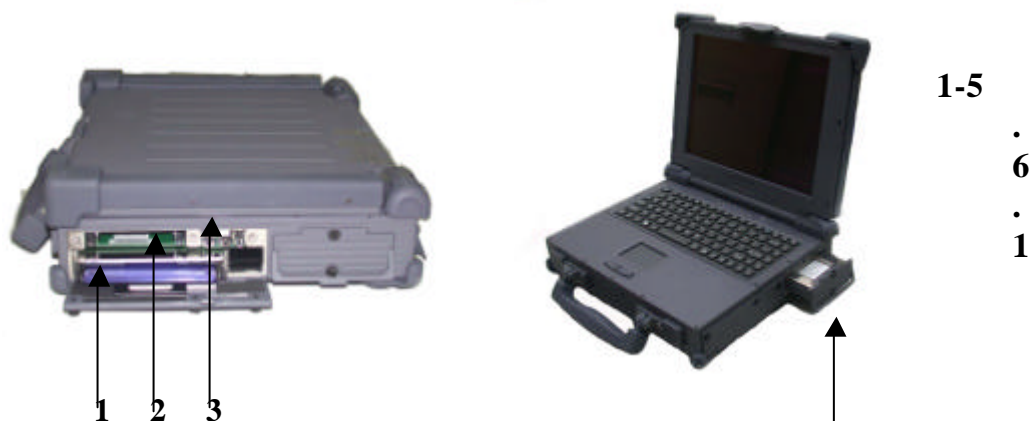
Figure 1-10 Diskette Drive and CD-ROM/DVD/COMBO /DVD RW PCMCIA Slot and Diskette Drive and CD-ROM/DVD /COMBO/DVD RW Door
