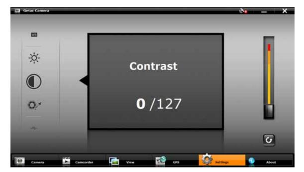
Along the left of the window are all the setting items. You can drag this area up or down to scroll through the items. The middle of the window displays the current item and setting value. To the right is the adjustment bar where you can tap or drag to change the setting value.
