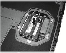
**CAUTION:** If the RAM module is difficult to insert or difficult to push down, do not force it. Check once more to ensure that the module is positioned correctly.
