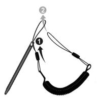
Insert the other loop end to the tether hole on the Tablet PC (as indicated by below). Then, insert the stylus end through the loop (as indicated by below) and pull it tight.
