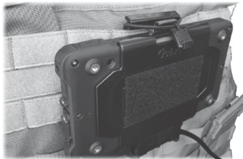
**NOTE:** The hinge of the mount might get loose after long time usage. Tighten the hex nut if this happens.
