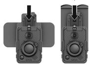
2. Slide the latch inwards to secure the camera to the mount.
