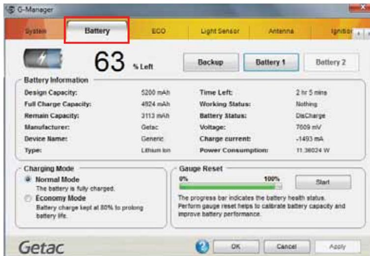
The battery items shown in the screen depend on your computer model. You may see up to three battery items (**Backup**, **Battery 1**, and **Battery 2**). Click a battery item to view the information of the selected battery. Batteries not installed in your computer are grayed-out.
