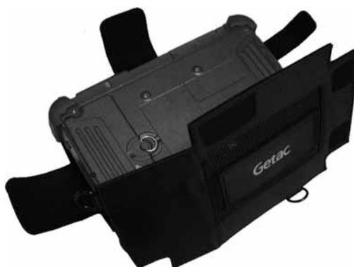
The hand strap allows you to firmly hold the Tablet PC by inserting your hand through the elastic band at the back.
