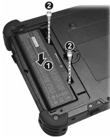
5. Replace the battery cover and turn the latch clockwise to the lock position.
