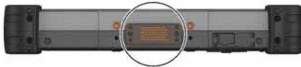
2. Connect the Docking Station to the docking connector.
