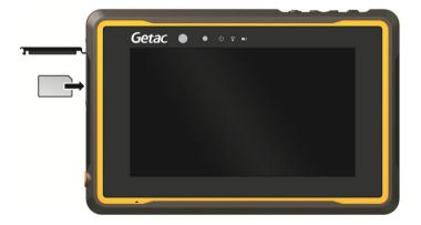
NOTE: To remove the SIM card, slightly push in the card to release it and then pull the card out of the slot.
