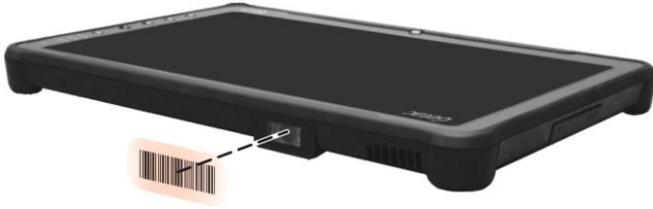
**NOTE:** If the code being scanned is highly reflective (e.g., laminated), it may be necessary to tilt the code +5° to prevent unwanted reflection.
