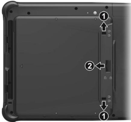
2. Pull the ribbon strip to lift the battery pack off the compartment.
