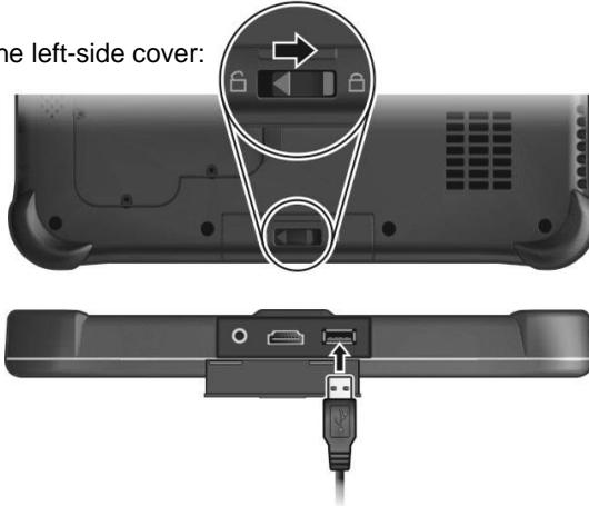
Select models have a second USB port, which supports USB 2.0 (transfer rate is 480 MB/s).
