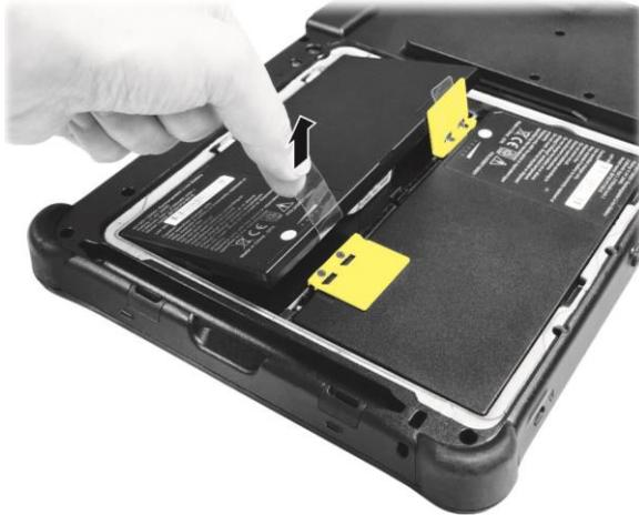
3. Fit another battery pack into place. Note the orientation of the battery pack. Hold the battery pack at an angle and insert its small tabs to the corresponding notches in the battery compartment. Then, lift the yellow protection sheet in the battery compartment and plug the battery connector.
