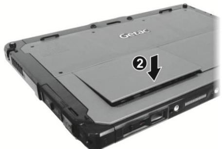
3. Slide the lock of the battery latch downward to the locked position.
