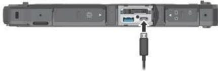
**CAUTION:** This port does not support USB Power Delivery. Never connect a power source to this port.
