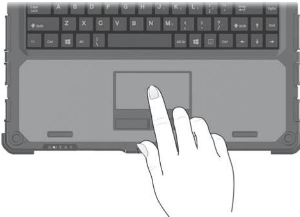
The touchpad consists of a rectangular pad (work surface) and a left and right buttons. To use the touchpad, place your forefinger or thumb on the pad. The rectangular pad acts like a miniature duplicate of your display. As you slide your fingertip across the pad, the pointer (also called cursor) on the screen moves accordingly. When your finger reaches the edge of the pad, simply relocate yourself by lifting the finger and placing it on the other side of the pad.
