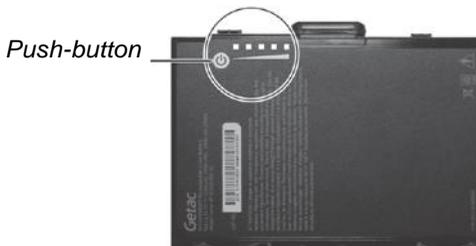
When the battery pack is not installed in the computer and you want to know the battery charge, you can press the push-button to see the number of LEDs that light up. Each LED represents 20% charge.
