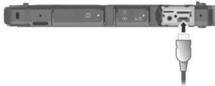
The Keyboard Dock has a VGA connector and a HDMI connector. Depending on the type of your monitor, plug the monitor's signal connector to the HDMI or VGA connector.
