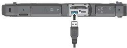
A connected device is charged by either external power (if the AC adapter is connected) or by the computer’s battery (if the AC adapter is not connected). In the latter case, charging will stop when the battery level gets low (20% capacity).
