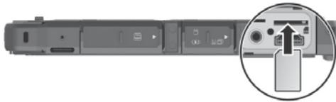
**NOTE:** To remove the micro-SIM card, just push in the card to release it and then pull it out.
