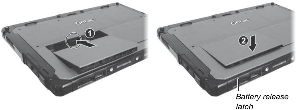
2. Slide the lock of the battery release latch downward to the locked position.
