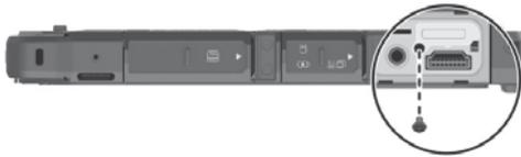
3. Noting the orientation, insert the micro-SIM card all the way into the slot.
