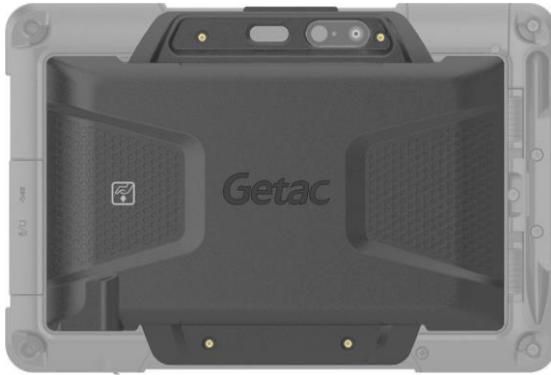
The second battery pack can be charged individually with the AC adapter when it is not attached to the Tablet PC. When attached, it will be charged after the main battery pack is charged.
