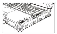
▶ Slide the battery pack all the way into the slot. Make sure to observe the correct orientation (the ribbon strip must face outward for future battery back removal).
